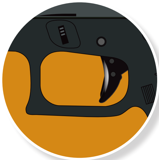
Reset Point The trigger resets at this point, and can be pressed again, without letting the trigger travel all the way forward to the rest position.
