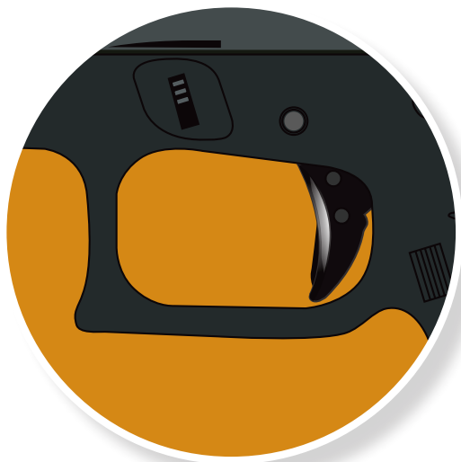
Break Point The point at which the striker is released, and the gun fires.
